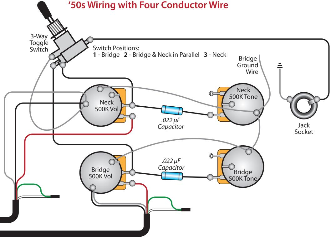
For normal humbucking wiring, solder green and white wires together,
